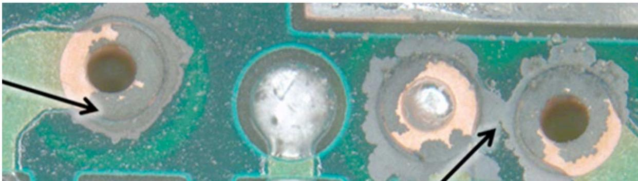
**Figure1: Copper corrosion created by copper creep.**
