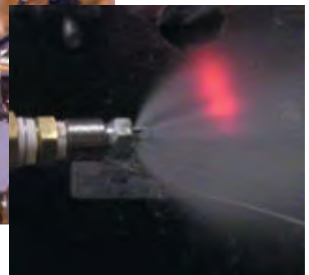
MeeFog™ nozzle droplet sizing with laser particle analyzer instrument.
