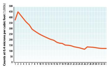
smoke odor. In addition, the SecureAire AQM-100 monitor displayed particle count reductions (0.4 micron size) of 74%.
