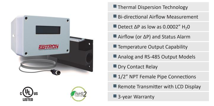
The EF-x2000-**B** is a unique measurement device that can detect very small pressure differentials (as low as  $0.0002'' H_2O$ ) between two adjacent spaces by sensing the airflow rate induced by the pressure gradient. The EF-x2000-B can be used to determine the airflow rate across fixed openings when a reference airflow rate is provided.
