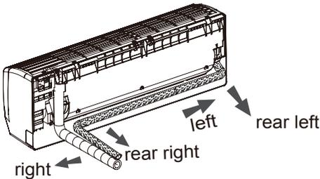
2. When select leading out the pipe from left or right, please cut off the corresponding hole on the bottom case.
