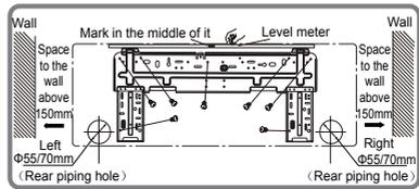
2. Open a piping hole with the diameter of  $\Phi 55$  or  $\Phi 70$  on the selected outlet pipe position. In order to drain smoothly, slant the piping hole on the wall slightly downward to the outdoor side with the gradient of 5-10°.
