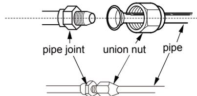
3. Adjust the torque force by referring to the following sheet. Place the open-end wrench on the pipe joint and place the torque wrench on the union nut. Tighten the union nut with torque wrench.
