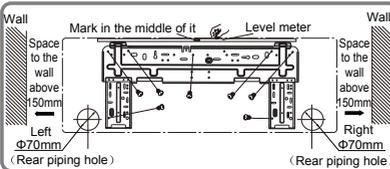
2. Open a piping hole with the diameter of  $\Phi 55$  or  $\Phi 70$  on the selected outlet pipe position. In order to drain smoothly, slant the piping hole on the wall slightly downward to the outdoor side with the gradient of  $5\text{-}10^\circ$ .
